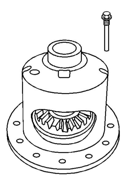
Fig. 17: Pinion Shaft Lock Bolt Courtesy of GENERAL MOTORS CORP.
