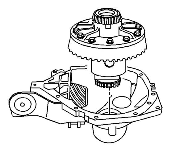
Fig. 124: Differential Case Assembly Courtesy of GENERAL MOTORS CORP.
