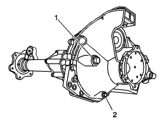
Fig. 28: Front Drive Axle Fill & Drain Plug Courtesy of GENERAL MOTORS CORP.
