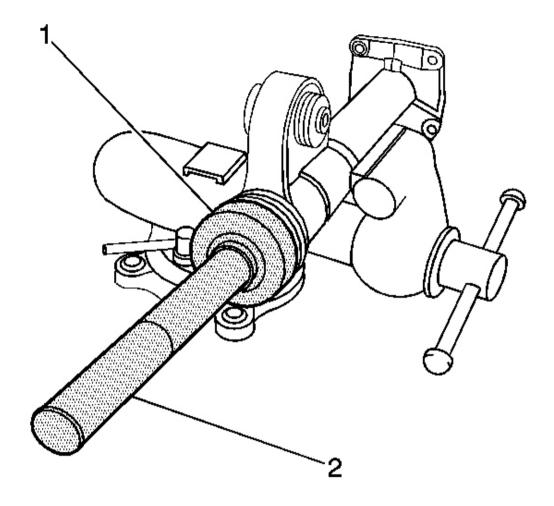
Fig. 133: Installing New Axle Shaft Seal Using J 45225 & J8092 Courtesy of GENERAL MOTORS CORP.
