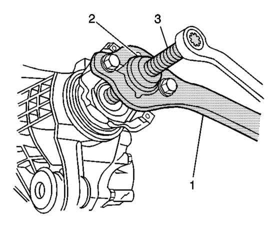
Fig. 54: Remove Pinion Yoke Using J 8614-2 & J 8614-3 Into J 8614-01 (8.25 Inch Axles) Courtesy of GENERAL MOTORS CORP.
