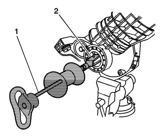
Fig. 73: Installing J 29369-2 Behind Inner Axle Shaft Seal Or Inner Axle Shaft Bearing Courtesy of GENERAL MOTORS CORP.
