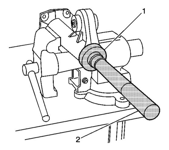
Fig. 47: Installing Bearing With Square Shoulder Using J 36609 & J 8092 Courtesy of GENERAL MOTORS CORP.
