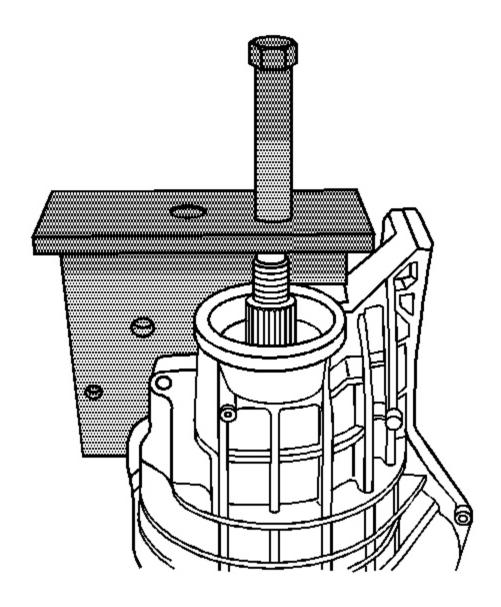
Fig. 84: Installing J 45765 To Left Side Differential Carrier Case Half Over Drive Pinion Courtesy of GENERAL MOTORS CORP.
