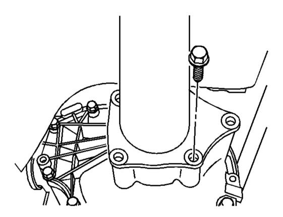
Fig. 41: Front Drive Inner Axle Shaft Housing Bolts Courtesy of GENERAL MOTORS CORP.
