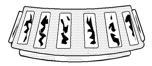
Fig. 12: Heat Discoloration Courtesy of GENERAL MOTORS CORP.
