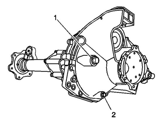
Fig. 27: Front Drive Axle Fill & Drain Plug Courtesy of GENERAL MOTORS CORP.
