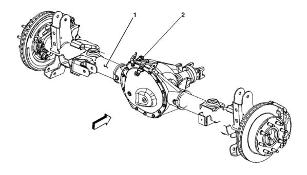
Fig. 2: Rear Differential Lock Actuator Component Views Courtesy of GENERAL MOTORS CORP.
