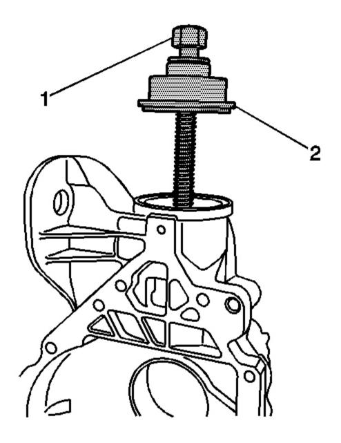
Fig. 88: Installing J 45754-2 & Forcing Screw Over Outer Pinion Bearing Cup Bore Courtesy of GENERAL MOTORS CORP.
