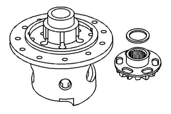
Fig. 21: Locking Differential Side Gear & Thrust Washer Courtesy of GENERAL MOTORS CORP.
