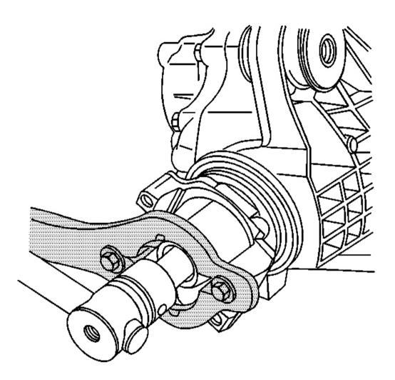
Fig. 56: Installing J 8614-01 Onto Pinion Yoke Courtesy of GENERAL MOTORS CORP.
