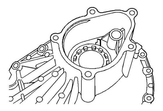
Fig. 127: Bending Right Side Differential Adjuster Nut Lock Tab Over Differential Adjuster Nut Sleeve
