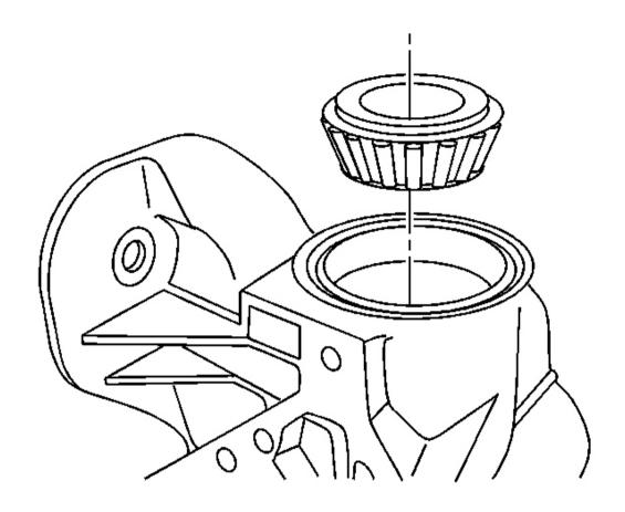
Fig. 114: Installing Outer Pinion Bearing Into Left Differential Carrier Case Half Courtesy of GENERAL MOTORS CORP.
