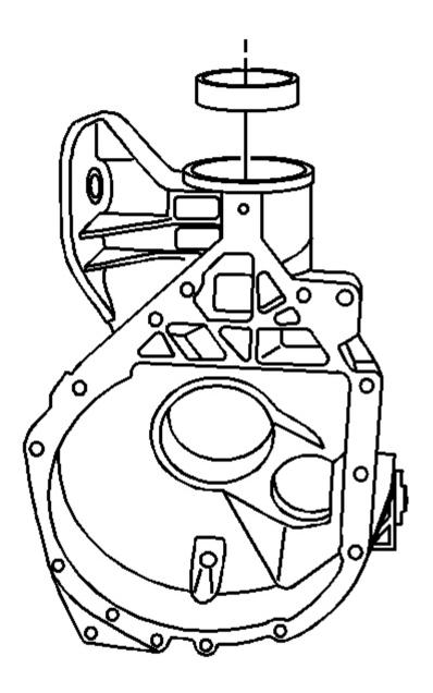
Fig. 105: Installing Outer Pinion Bearing Cup Into Outer Pinion Bearing Cup Bore Courtesy of GENERAL MOTORS CORP.
