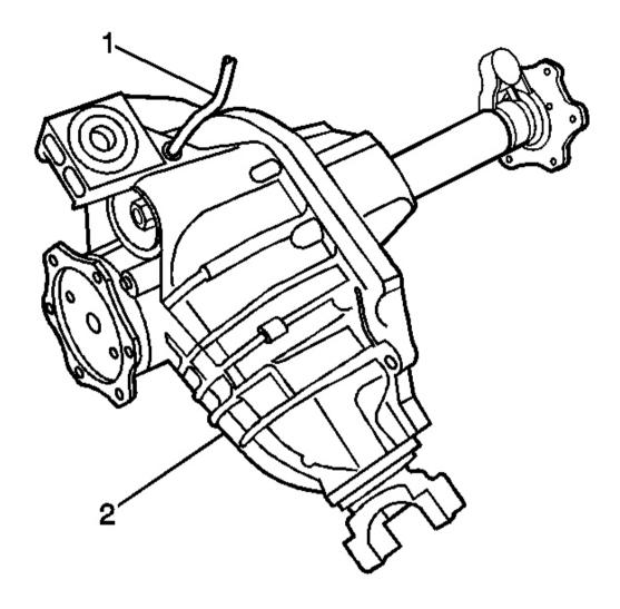
Fig. 32: Identifying Vent Hose & Differential Carrier Case Assembly Courtesy of GENERAL MOTORS CORP.
