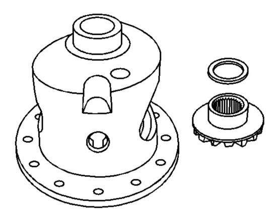
Fig. 27: Differential Side Gears & Thrust Washers Courtesy of GENERAL MOTORS CORP.
