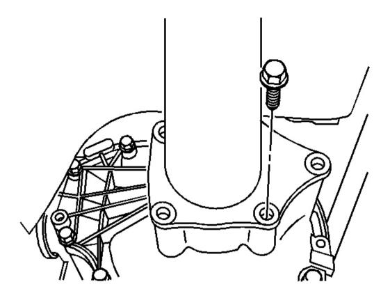
Fig. 40: Front Drive Inner Axle Shaft Housing Bolts Courtesy of GENERAL MOTORS CORP.
