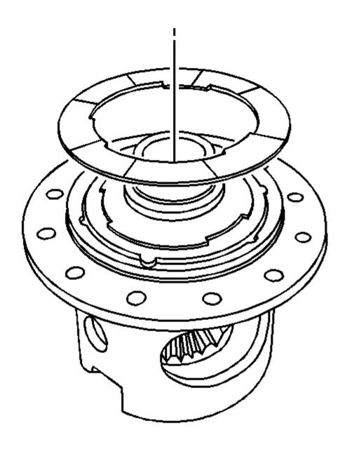
Fig. 42: Locking Differential Coil Plate Courtesy of GENERAL MOTORS CORP.
