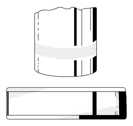
Fig. 23: Misalignment Courtesy of GENERAL MOTORS CORP.
