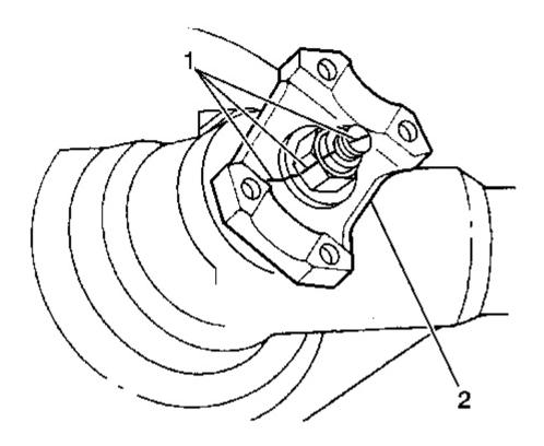
Fig. 52: Scribing Line On Pinion Shaft & Pinion Yoke Courtesy of GENERAL MOTORS CORP.
