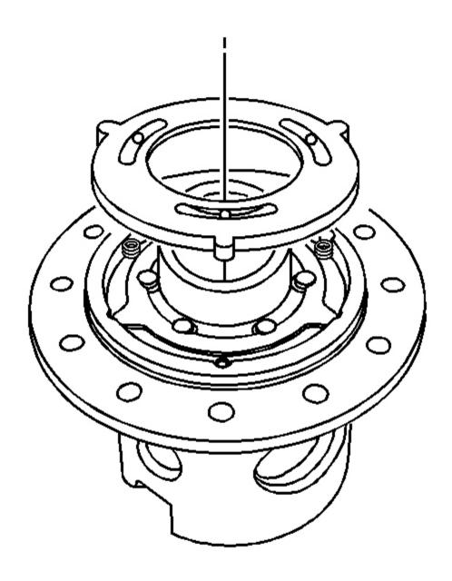
Fig. 14: Inboard Locking Differential Ball Bearing Plate Courtesy of GENERAL MOTORS CORP.
