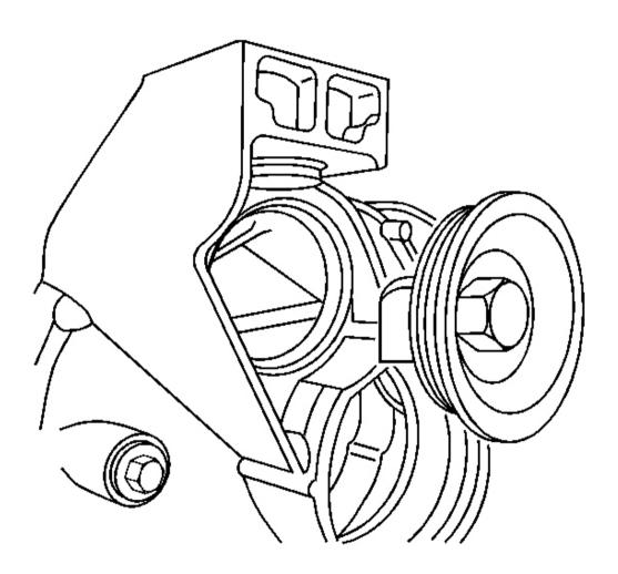
Fig. 131: Differential Carrier Assembly & Hole Plug Courtesy of GENERAL MOTORS CORP.
