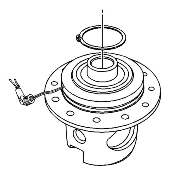
Fig. 4: Differential Bearing Retainer Courtesy of GENERAL MOTORS CORP.
