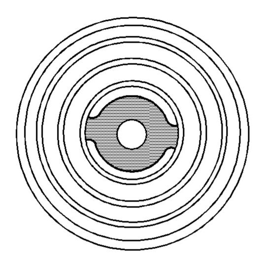
Fig. 86: Installing J 45754-3 Over Inner Pinion Bearing Cup Courtesy of GENERAL MOTORS CORP.
