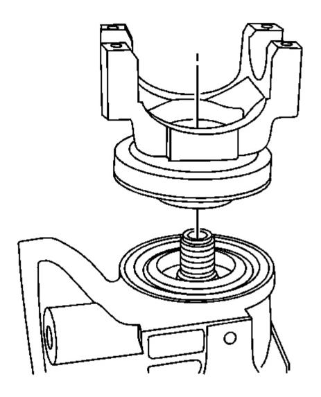
Fig. 117: Installing Pinion Yoke Courtesy of GENERAL MOTORS CORP.
