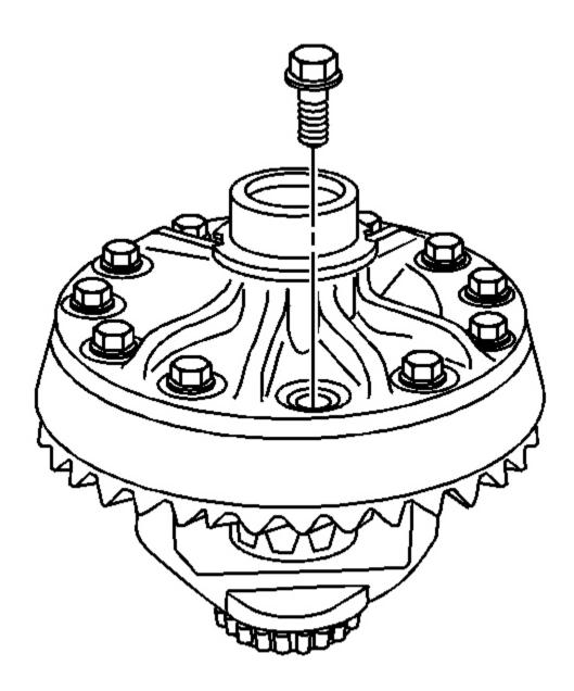
Fig. 92: Identifying Ring Gear Bolts Courtesy of GENERAL MOTORS CORP.
