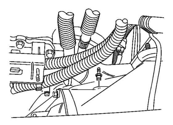
Fig. 35: Front Drive Axle Vent Hose Connector Courtesy of GENERAL MOTORS CORP.
