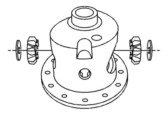
Fig. 28: Differential Pinion Gears & Thrust Washers Courtesy of GENERAL MOTORS CORP.
