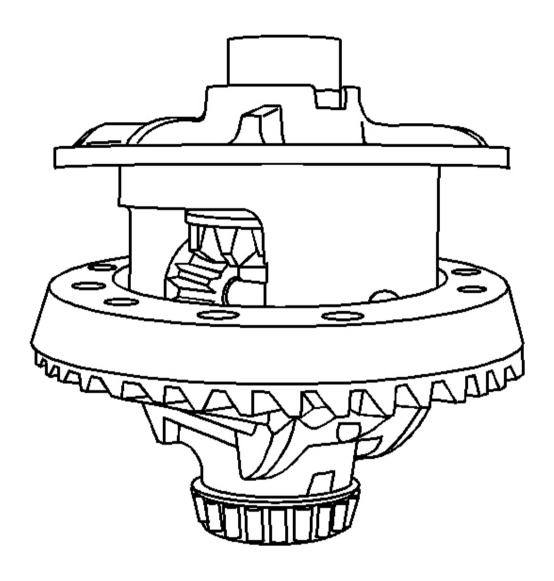
Fig. 102: Installing Ring Gear Onto Differential Case Courtesy of GENERAL MOTORS CORP.
