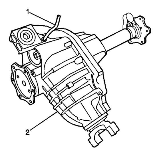
Fig. 65: Identifying Vent Hose & Differential Carrier Case Assembly Courtesy of GENERAL MOTORS CORP.
