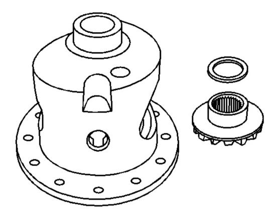
Fig. 33: Differential Side Gears & Thrust Washers Courtesy of GENERAL MOTORS CORP.
