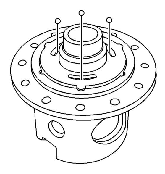
Fig. 40: Locking Differential Ball Bearings Courtesy of GENERAL MOTORS CORP.
