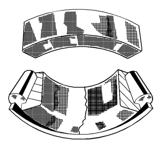
Fig. 14: Cracked Inner Race Courtesy of GENERAL MOTORS CORP.
