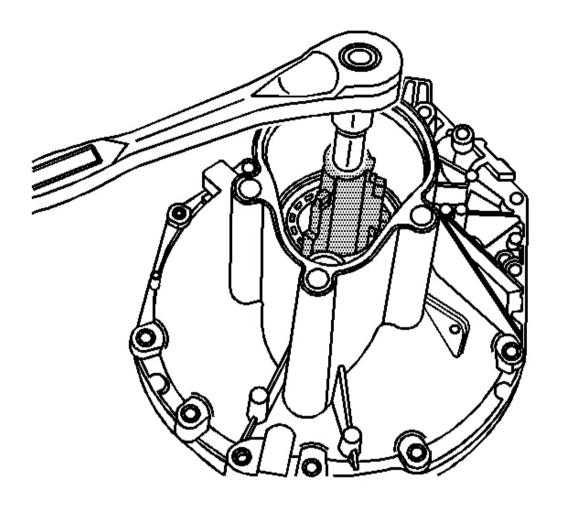
Fig. 80: Remove Right Side Differential Side Bearing Cup, Differential Bearing Adjuster Nut & Differential Bearing Adjuster Sleeve Courtesy of GENERAL MOTORS CORP.
