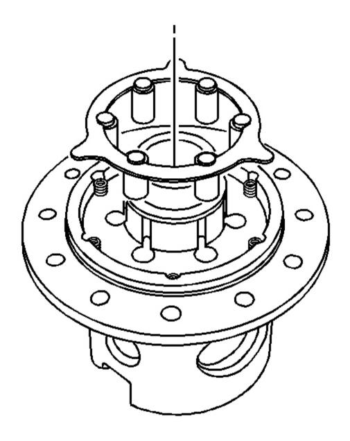
Fig. 15: Locking Differential Clutch Spring Retainer & Differential Carrier Lock Pins Courtesy of GENERAL MOTORS CORP.
