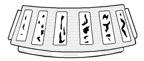
Fig. 15: Fatigue Spalling Courtesy of GENERAL MOTORS CORP.
