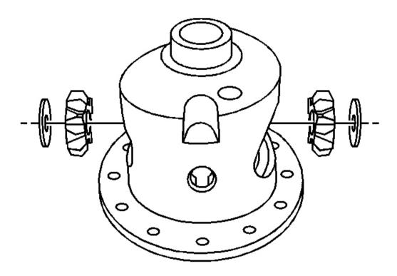
Fig. 99: Differential Pinion Gears & Thrust Washers Courtesy of GENERAL MOTORS CORP.
