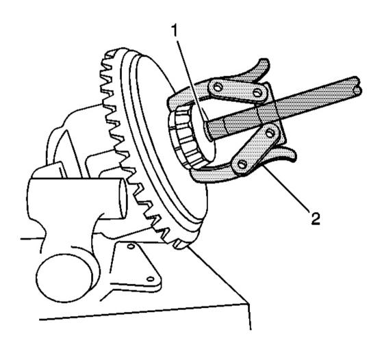
Fig. 91: Removing Differential Side Bearings Courtesy of GENERAL MOTORS CORP.
