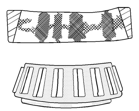
Fig. 2: Abrasive Roller Wear Courtesy of GENERAL MOTORS CORP.
