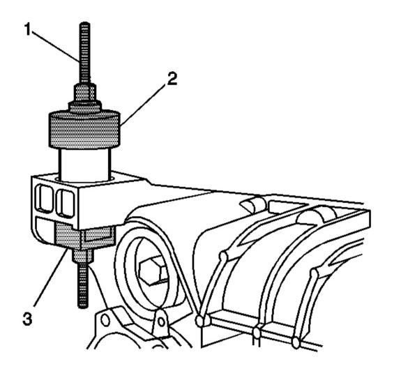
Fig. 59: Installing J 45755-2, J 45755-1, Forcing Screw, Bearing & Washers Over Differential Carrier Assembly Bushing Courtesy of GENERAL MOTORS CORP.
