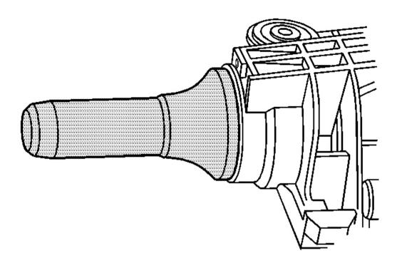
Fig. 55: Installing Oil Seal Using J 36366 Courtesy of GENERAL MOTORS CORP.
