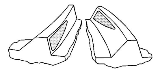
Fig. 140: Drive Side Heel - Coast Side Toe Contact Pattern Courtesy of GENERAL MOTORS CORP.
