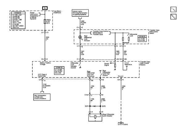
Fig. 1: Differential Lock Schematics
