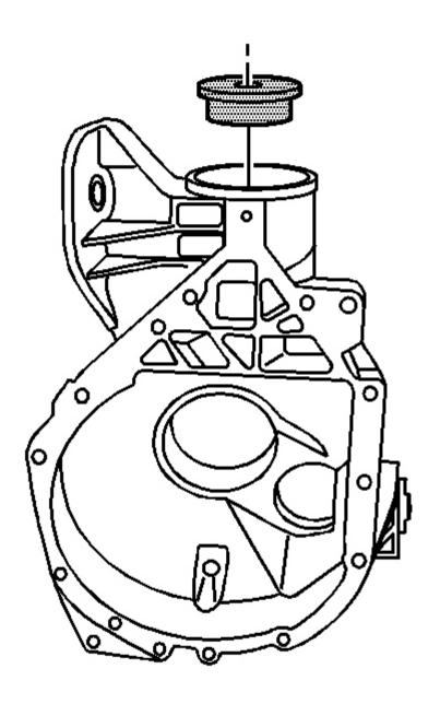
Fig. 106: Installing J 45754-1 Over Outer Pinion Bearing Cup Courtesy of GENERAL MOTORS CORP.
