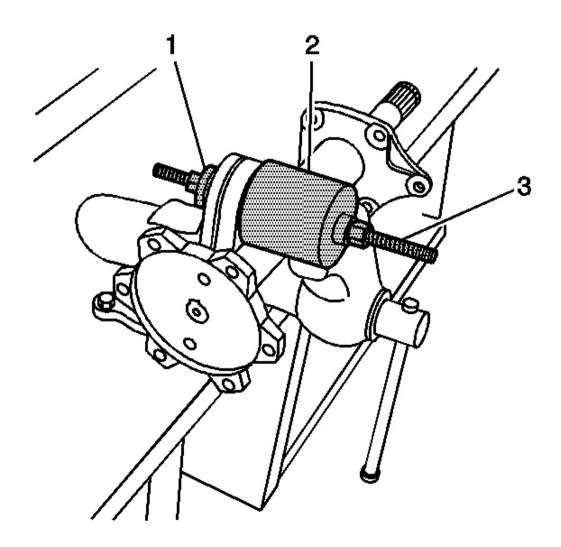
Fig. 60: Installing J 45755-2, J 45755-1, Forcing Screw, Bearing & Washers Over Inner Shaft Housing Bushing
