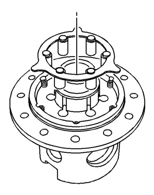
Fig. 38: Locking Differential Clutch Spring Retainer & Differential Carrier Lock Pins Courtesy of GENERAL MOTORS CORP.
