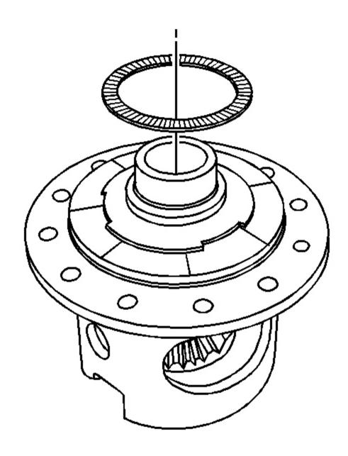
Fig. 10: Removing Differential Bearing Assembly Courtesy of GENERAL MOTORS CORP.
