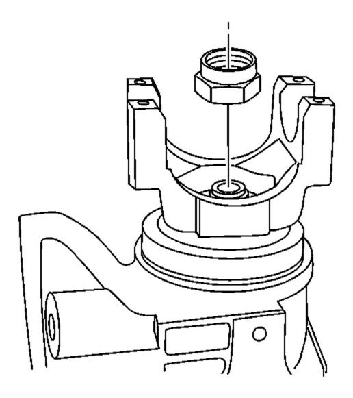
Fig. 119: Installing New Pinion Nut
