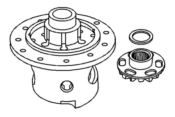
Fig. 22: Locking Differential Side Gear & Thrust Washer Courtesy of GENERAL MOTORS CORP.
