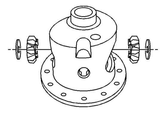
Fig. 34: Differential Pinion Gears & Thrust Washers Courtesy of GENERAL MOTORS CORP.
