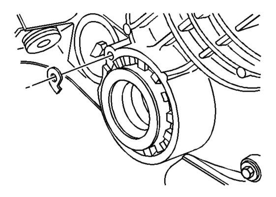
Fig. 79: Differential Adjuster Nut Lock Courtesy of GENERAL MOTORS CORP.
