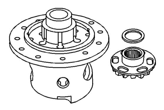
Fig. 32: Locking Differential Side Gear & Thrust Washer Courtesy of GENERAL MOTORS CORP.
