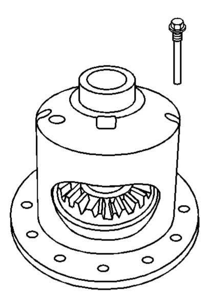
Fig. 101: Pinion Shaft Lock Bolt Courtesy of GENERAL MOTORS CORP.
