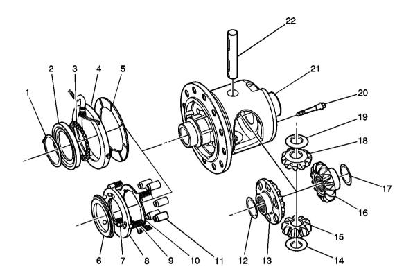
Fig. 3: Locking Differential Component Views Courtesy of GENERAL MOTORS CORP.
