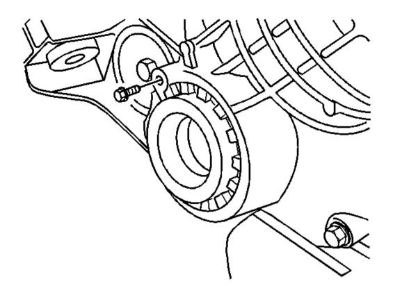
Fig. 78: Differential Adjuster Nut Lock Bolt Courtesy of GENERAL MOTORS CORP.
