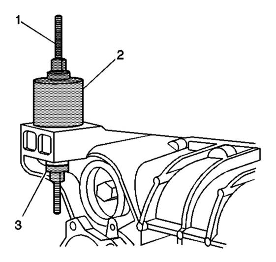
Fig. 90: Installing J 45755-3, J 45755-4, Forcing Screw, Bearing & Washers Over Differential Carrier Assembly
