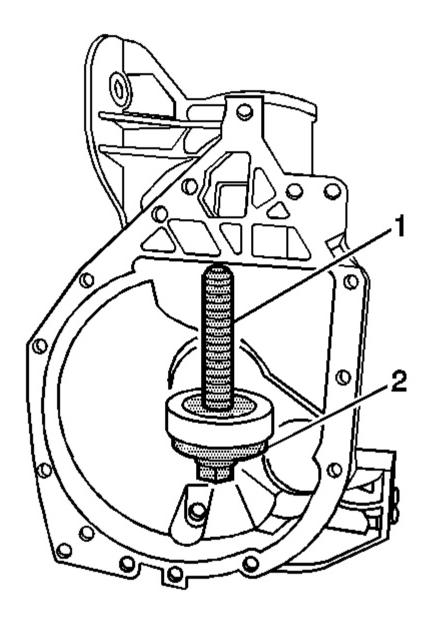
Fig. 108: Installing Inner Pinion Bearing Cup Onto J 45754-2 & Forcing Screw Courtesy of GENERAL MOTORS CORP.
