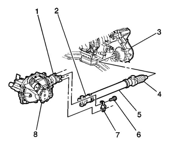
Fig. 50: Propeller Shaft & Front Axle Pinion Yoke Courtesy of GENERAL MOTORS CORP.
