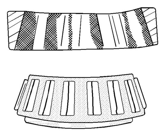
Fig. 16: Brinelling Courtesy of GENERAL MOTORS CORP.
