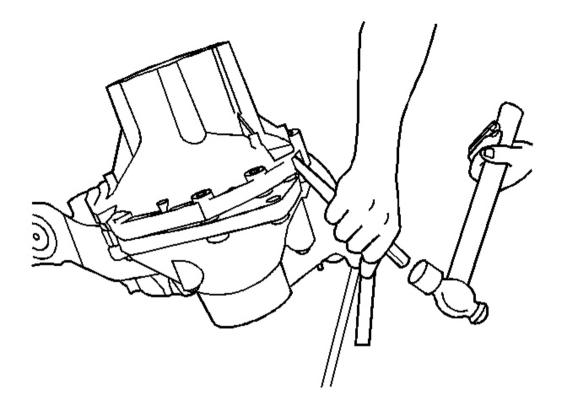
Fig. 76: Separating Left & Right Carrier Case Half By Tapping On Carrier Case Lugs With Hammer Courtesy of GENERAL MOTORS CORP.
