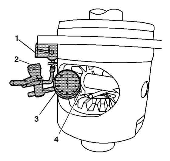
Fig. 31: Measuring Backlash Of Pinion Gear Closest To Pinion Shaft Lock Bolt & Differential Side Gear
