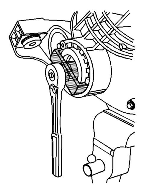
Fig. 125: Turning Left Side Differential Adjuster Nut Sleeve Using J 36615 Courtesy of GENERAL MOTORS CORP.
