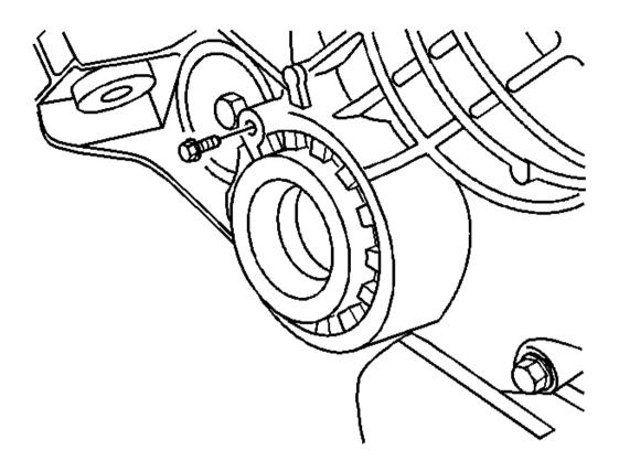
Fig. 129: Differential Adjuster Nut Lock Bolt Courtesy of GENERAL MOTORS CORP.
