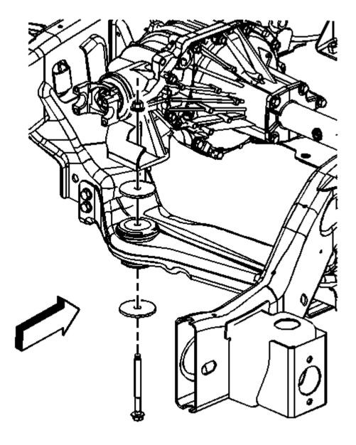
Fig. 64: Differential Carrier Assembly Left & Right Side Axle Mount Bolts & Nuts Courtesy of GENERAL MOTORS CORP.
