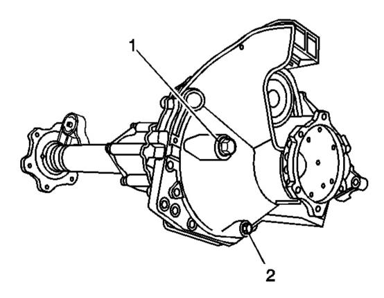
Fig. 26: Front Drive Axle Fill & Drain Plug
