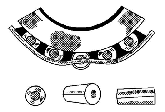
Fig. 6: Bent Cage Courtesy of GENERAL MOTORS CORP.
