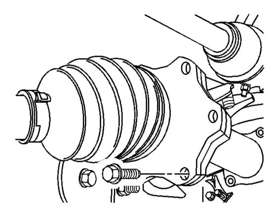
Fig. 37: Wheel Drive Shaft Inboard Flange Bolt - Front Drive Axle Courtesy of GENERAL MOTORS CORP.
