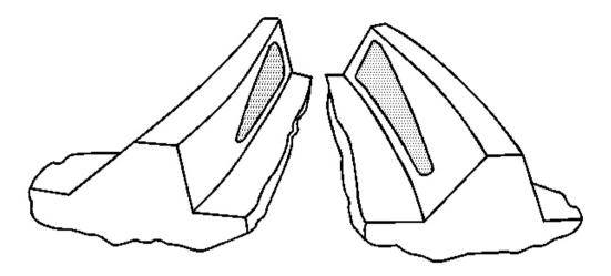
Fig. 143: Drive Side Toe - Coast Side Toe Contact Pattern Courtesy of GENERAL MOTORS CORP.
