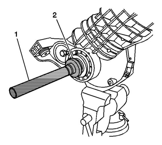
Fig. 123: Installing Left Side Axle Shaft Bearing Using J 36609 & J 8092 Courtesy of GENERAL MOTORS CORP.
