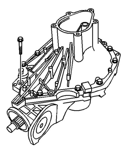
Fig. 75: Removing Differential Carrier Assembly Bolts Courtesy of GENERAL MOTORS CORP.
