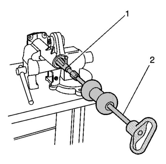
Fig. 45: Installing J 29369-02 Behind Inner Axle Shaft Seal
