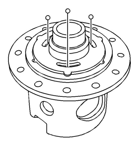
Fig. 13: Locking Differential Ball Bearings Courtesy of GENERAL MOTORS CORP.
