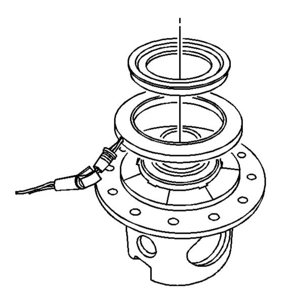
Fig. 43: Differential Bearing Race Courtesy of GENERAL MOTORS CORP.
