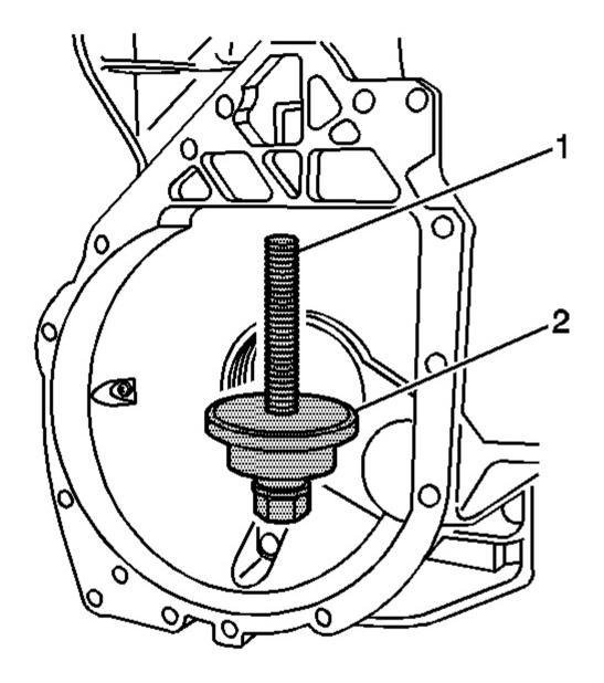
Fig. 107: Installing Forcing Screw & J 45754-2 Into Inner Pinion Bearing Cup Bore Courtesy of GENERAL MOTORS CORP.
