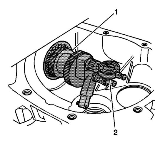
Fig. 111: Adjusting J 29763 To Differential Bearing Bore Courtesy of GENERAL MOTORS CORP.
