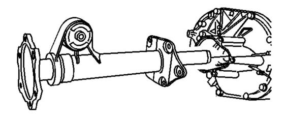
Fig. 67: Inner Axle Housing & Inner Axle Shaft Courtesy of GENERAL MOTORS CORP.
