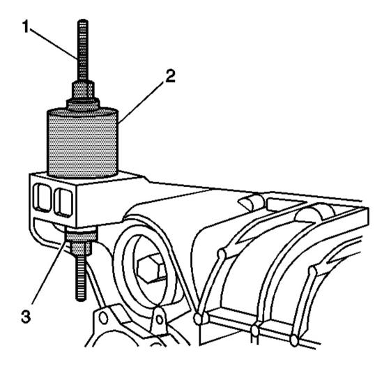
Fig. 58: Installing J 45755-3, J 45755-4, Forcing Screw, Bearing & Washers Over Differential Carrier Assembly
