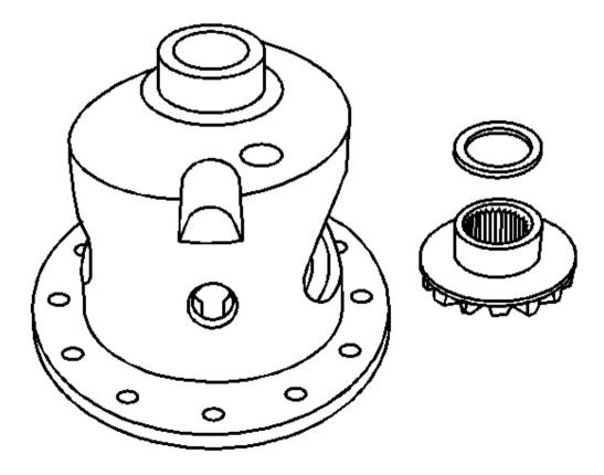
Fig. 98: Differential Side Gears & Thrust Washers
