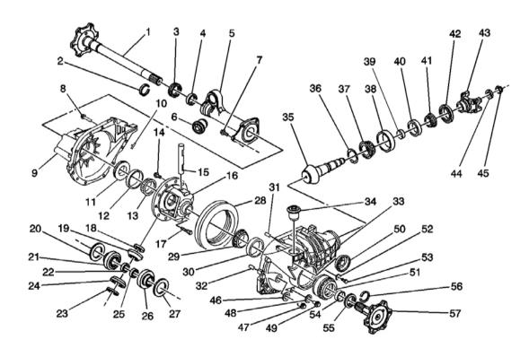
Fig. 1: Front Drive Axle Component Views Courtesy of GENERAL MOTORS CORP.
