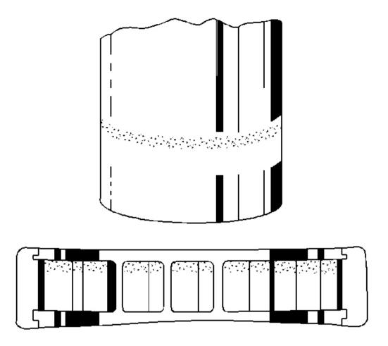
Fig. 21: Single Edge Pitting Courtesy of GENERAL MOTORS CORP.
