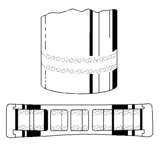
Fig. 22: Double Edge Pitting Courtesy of GENERAL MOTORS CORP.
