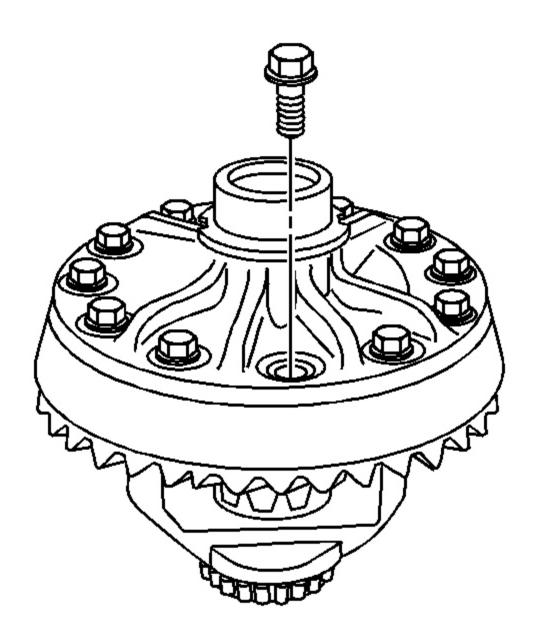
Fig. 103: Identifying Ring Gear Bolts Courtesy of GENERAL MOTORS CORP.
