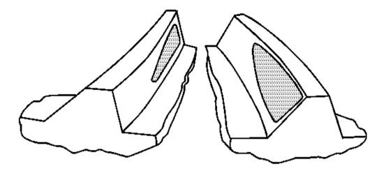
Fig. 141: Drive Side Toe - Coast Side Heel Contact Pattern Courtesy of GENERAL MOTORS CORP.
