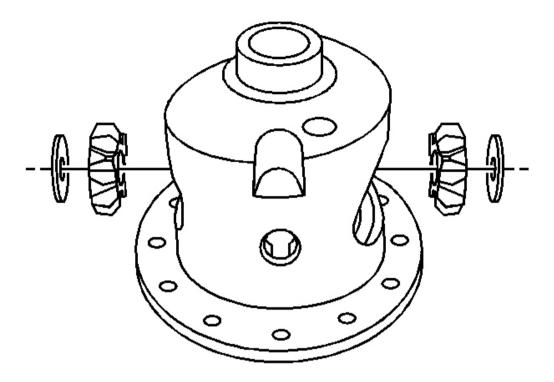
Fig. 96: Differential Pinion Gears & Thrust Washers Courtesy of GENERAL MOTORS CORP.
