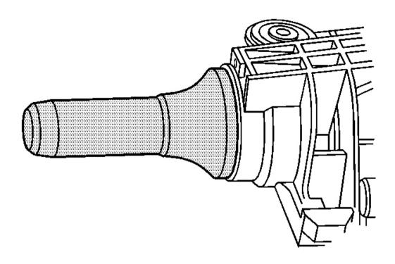
Fig. 115: Installing Oil Seal Using J 36366 Courtesy of GENERAL MOTORS CORP.
