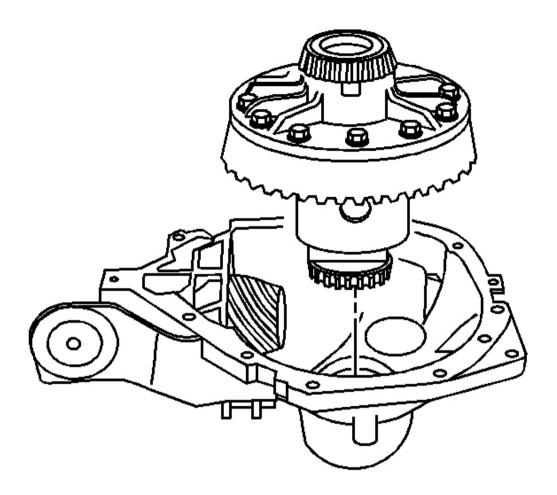
Fig. 77: Differential Case Assembly Courtesy of GENERAL MOTORS CORP.
