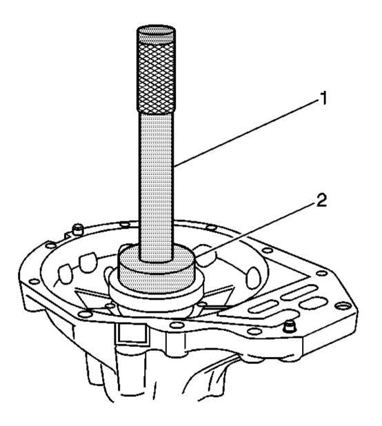
Fig. 122: Installing Right Side Differential Case Side Bearing Cup Into Differential Carrier Case Using J 36603 & J 8092 Courtesy of GENERAL MOTORS CORP.
