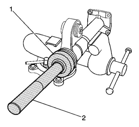
Fig. 48: Installing New Axle Shaft Seal Using J 45225 & J8092 Courtesy of GENERAL MOTORS CORP.
