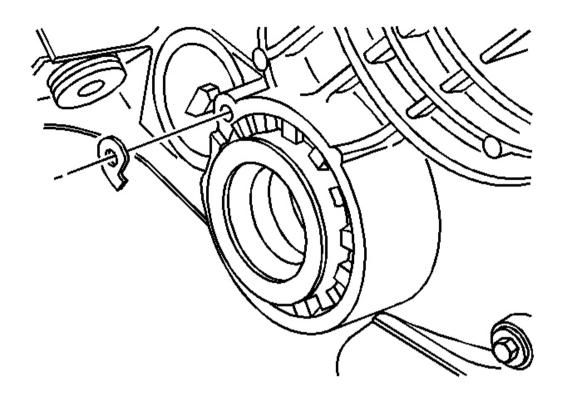
Fig. 128: Differential Adjuster Nut Lock Courtesy of GENERAL MOTORS CORP.
