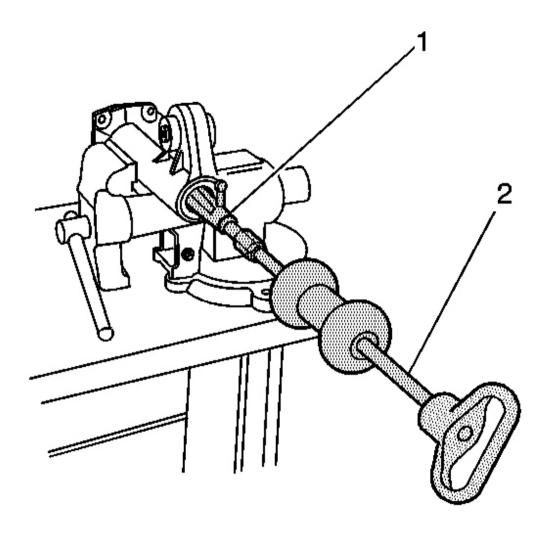
Fig. 70: Installing J 29369-02 Behind Inner Axle Shaft Seal Courtesy of GENERAL MOTORS CORP.
