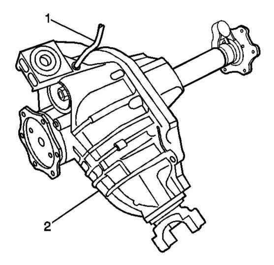
Fig. 62: Identifying Vent Hose & Differential Carrier Case Assembly Courtesy of GENERAL MOTORS CORP.
