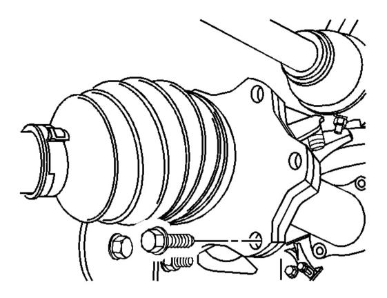
Fig. 43: Wheel Drive Shaft Inboard Flange Bolt - Front Drive Axle Courtesy of GENERAL MOTORS CORP.
