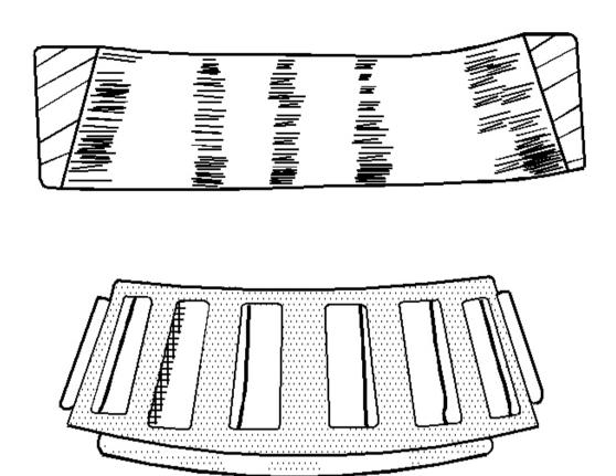
Fig. 7: Cage Wear Courtesy of GENERAL MOTORS CORP.
