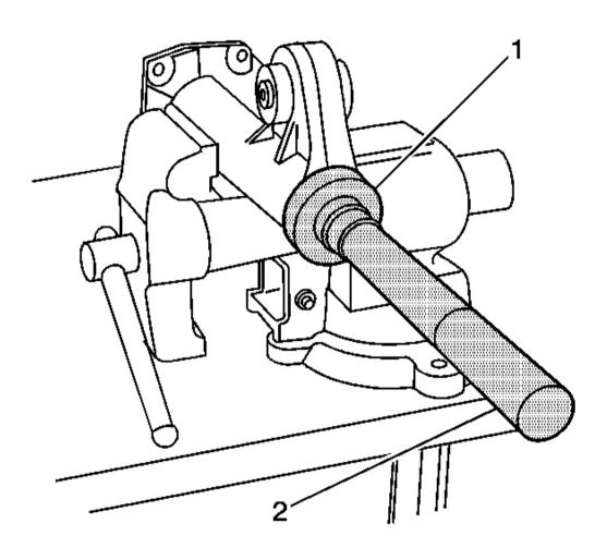
Fig. 132: Installing Bearing With Square Shoulder Using J 36609 & J 8092 Courtesy of GENERAL MOTORS CORP.
