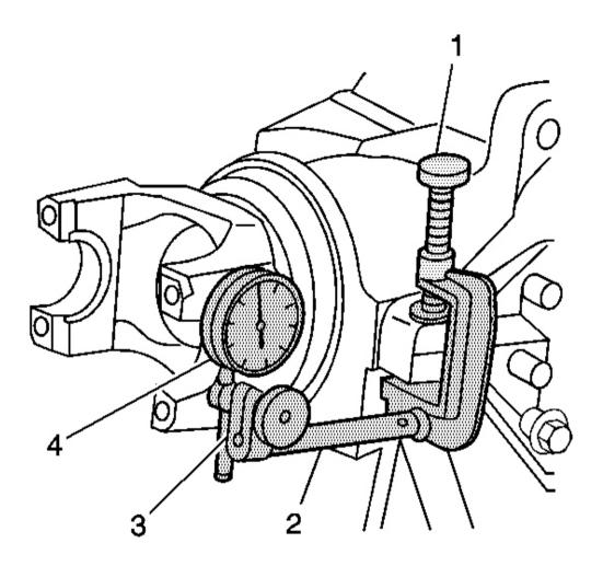
Fig. 126: Installing J 8001-1, J 8001-2 & J 8001-3 Courtesy of GENERAL MOTORS CORP.
