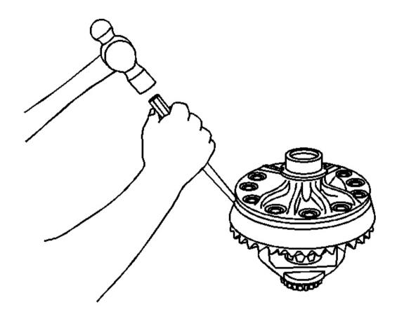
Fig. 93: Removing Ring Gear From Differential Case Courtesy of GENERAL MOTORS CORP.
