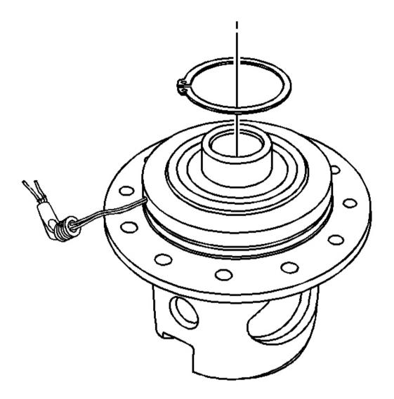
Fig. 7: Differential Bearing Retainer Courtesy of GENERAL MOTORS CORP.
