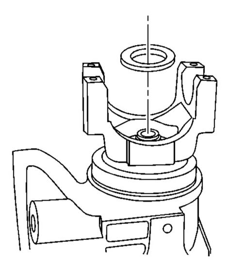
Fig. 118: Installing Washer Courtesy of GENERAL MOTORS CORP.
