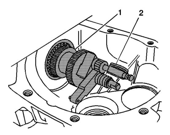
Fig. 112: Grasping J 36601 By Flats & Moving J 36601 Out Of Differential Side Bearing Bore Courtesy of GENERAL MOTORS CORP.
