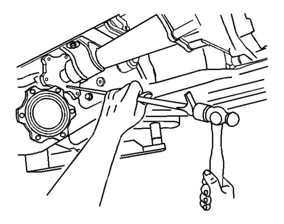
Fig. 38: Disconnecting Front Drive Inner Axle Shaft From Differential Case Side Gear Courtesy of GENERAL MOTORS CORP.
