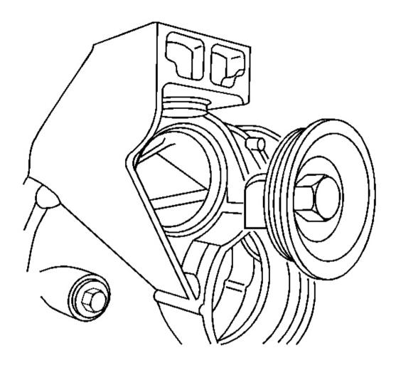
Fig. 74: Differential Carrier Assembly & Hole Plug Courtesy of GENERAL MOTORS CORP.
