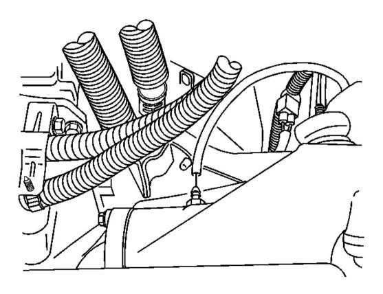
Fig. 33: Front Drive Axle Vent Hose & Vent Hose Connector Courtesy of GENERAL MOTORS CORP.
