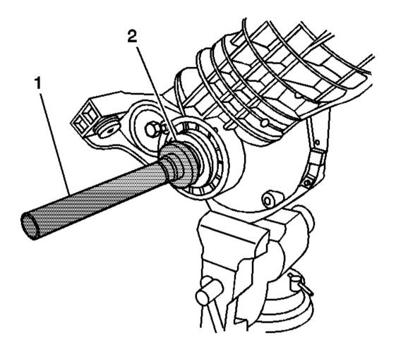
Fig. 49: Installing Left Side Axle Shaft Bearing Using J 36609 & J 8092 Courtesy of GENERAL MOTORS CORP.
