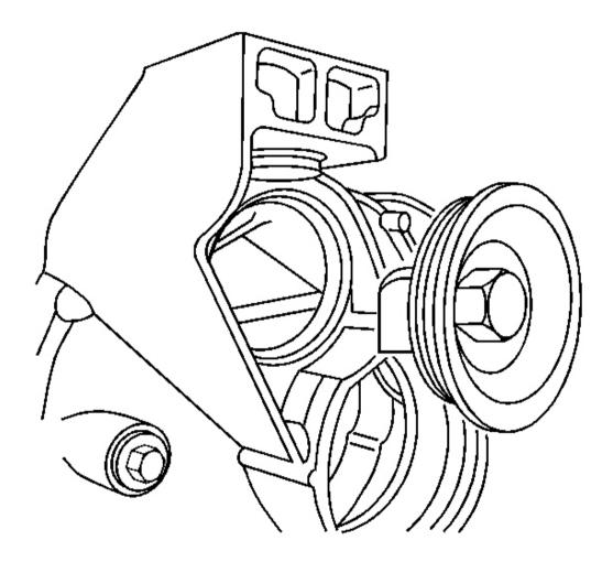
Fig. 29: Differential Carrier Assembly & Hole Plug Courtesy of GENERAL MOTORS CORP.
