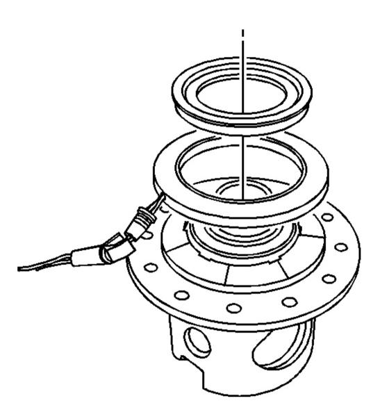
Fig. 5: Differential Bearing Race Courtesy of GENERAL MOTORS CORP.
