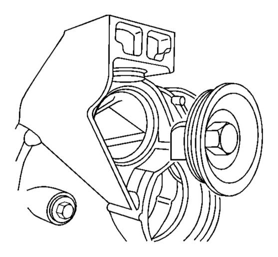
Fig. 30: Differential Carrier Assembly & Hole Plug Courtesy of GENERAL MOTORS CORP.
