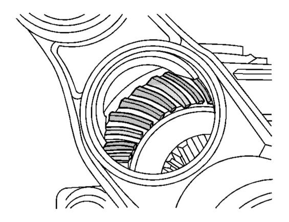
Fig. 138: Applying Gear Marking Compound GM P/N 1052351 Courtesy of GENERAL MOTORS CORP.
