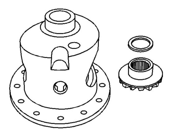
Fig. 20: Differential Side Gears & Thrust Washers Courtesy of GENERAL MOTORS CORP.
