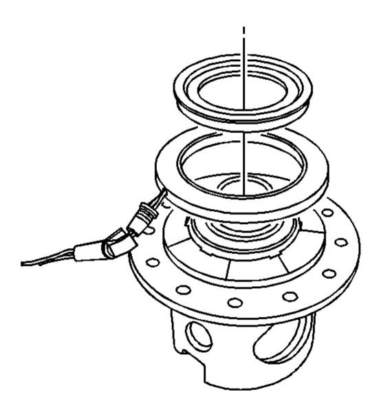
Fig. 6: Differential Bearing Race Courtesy of GENERAL MOTORS CORP.
