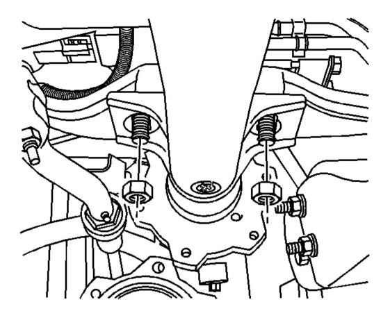
Fig. 42: Front Drive Inner Axle Shaft Housing Nuts Courtesy of GENERAL MOTORS CORP.
