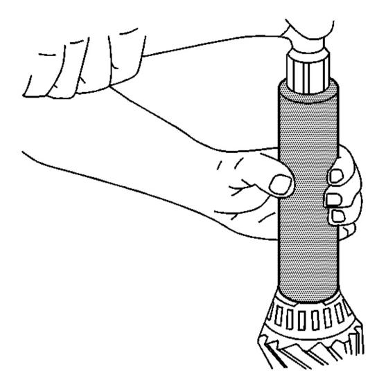
Fig. 113: Installing Inner Pinion Bearing Courtesy of GENERAL MOTORS CORP.
