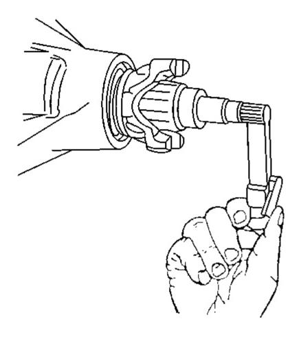
Fig. 51: Measuring Pinion Rotation Torque - Front Axle Courtesy of GENERAL MOTORS CORP.
