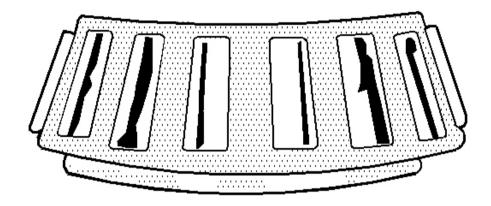
Fig. 13: Misalignment Courtesy of GENERAL MOTORS CORP.
