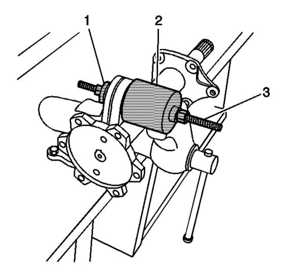
Fig. 68: Installing J 45755-2, J 45755-1, Forcing Screw, Bearing & Washers Over Inner Shaft Housing Bushing Courtesy of GENERAL MOTORS CORP.
