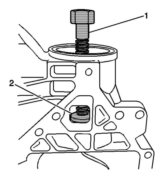
Fig. 87: Installing Forcing Screw Of J 45754 Into J 45754-3 Courtesy of GENERAL MOTORS CORP.
