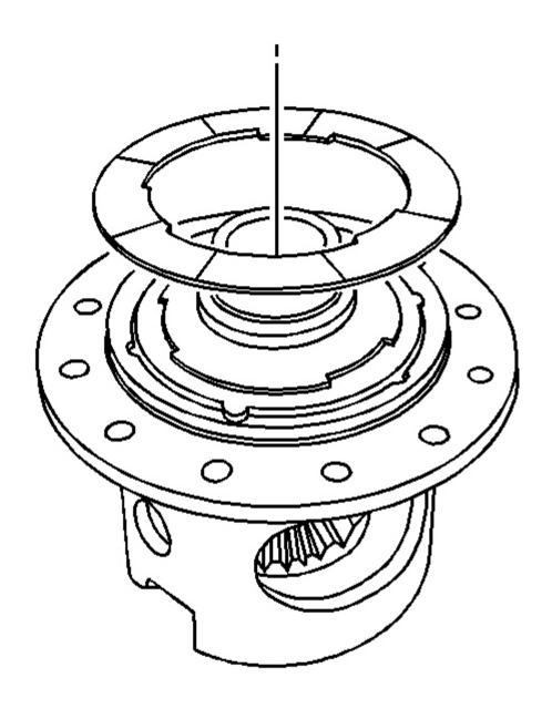
Fig. 11: Locking Differential Coil Plate Courtesy of GENERAL MOTORS CORP.
