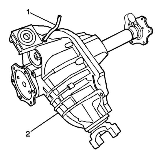
Fig. 31: Identifying Vent Hose & Differential Carrier Case Assembly Courtesy of GENERAL MOTORS CORP.
