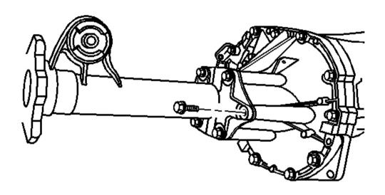
Fig. 136: Inner Axle Shaft Housing & Differential Carrier Assembly Bolts Courtesy of GENERAL MOTORS CORP.
