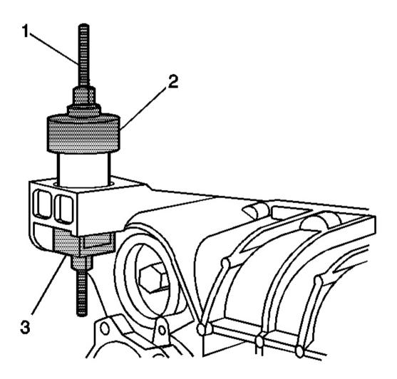
Fig. 130: Installing J 45755-2, J 45755-1, Forcing Screw, Bearing & Washers Over Differential Carrier Assembly Bushing Courtesy of GENERAL MOTORS CORP.
