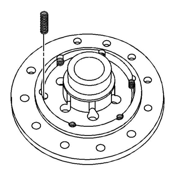
Fig. 16: Locking Differential Clutch Springs Courtesy of GENERAL MOTORS CORP.
