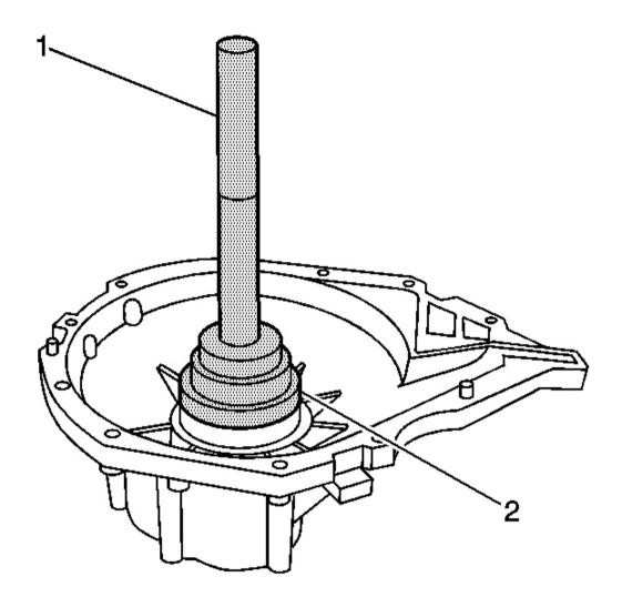
Fig. 121: Driving Right Side Differential Adjuster Nut Assembly & New Adjuster Lock Nut Tab Into Differential Carrier Case Half Using J 36609 & J8092 Courtesy of GENERAL MOTORS CORP.
