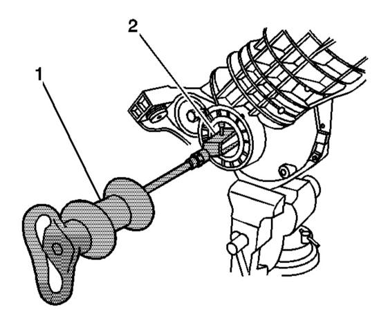
Fig. 72: Installing J 2619-01 & J 29369-2 Courtesy of GENERAL MOTORS CORP.
