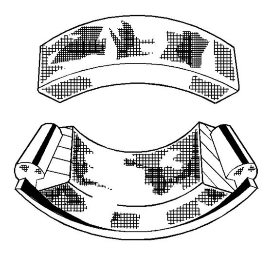
Fig. 10: Smears Courtesy of GENERAL MOTORS CORP.
