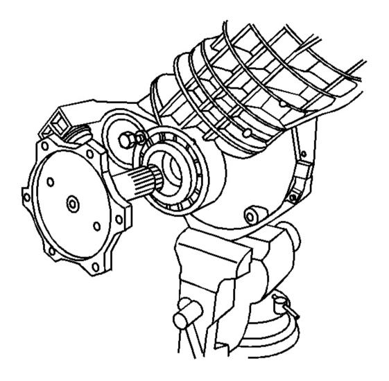
Fig. 71: Removing Left Side Inner Axle Shaft Courtesy of GENERAL MOTORS CORP.
