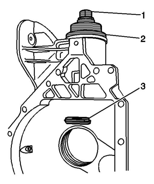
Fig. 89: Installing J 45754-4 Into Pinion Bearing Bore Behind Outer Pinion Bearing Cup Courtesy of GENERAL MOTORS CORP.
