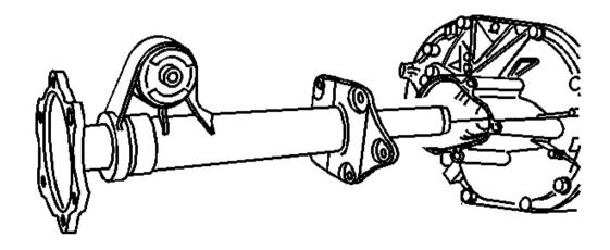
Fig. 135: Inner Axle Housing & Inner Axle Shaft
