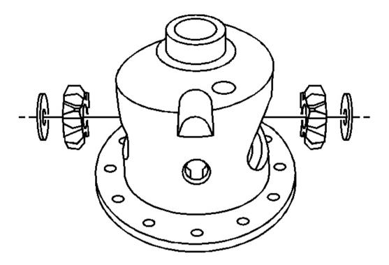
Fig. 23: Differential Pinion Gears & Thrust Washers Courtesy of GENERAL MOTORS CORP.
