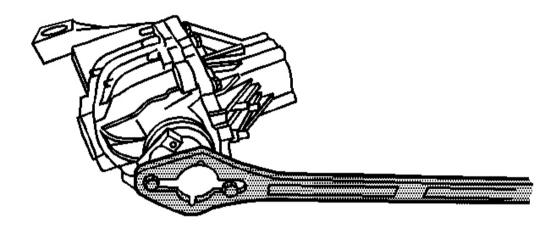
Fig. 120: Installing J 8614-01 Onto Pinion Yoke Courtesy of GENERAL MOTORS CORP.
