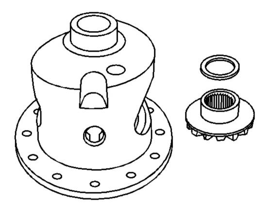
Fig. 97: Differential Side Gears & Thrust Washers Courtesy of GENERAL MOTORS CORP.
