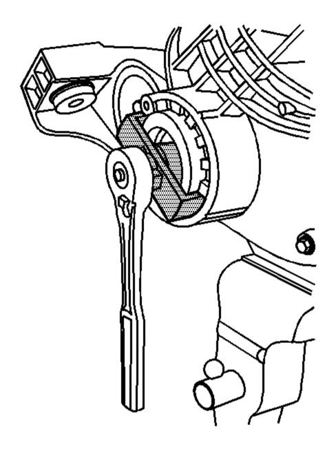
Fig. 81: Turning Left Side Differential Adjuster Nut Sleeve Using J 36615 Courtesy of GENERAL MOTORS CORP.
