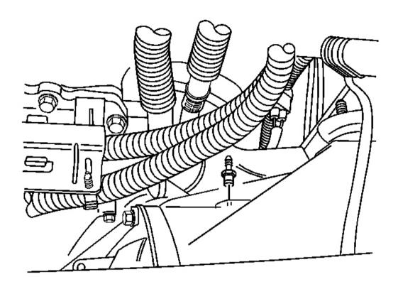
Fig. 34: Front Drive Axle Vent Hose Connector Courtesy of GENERAL MOTORS CORP.
