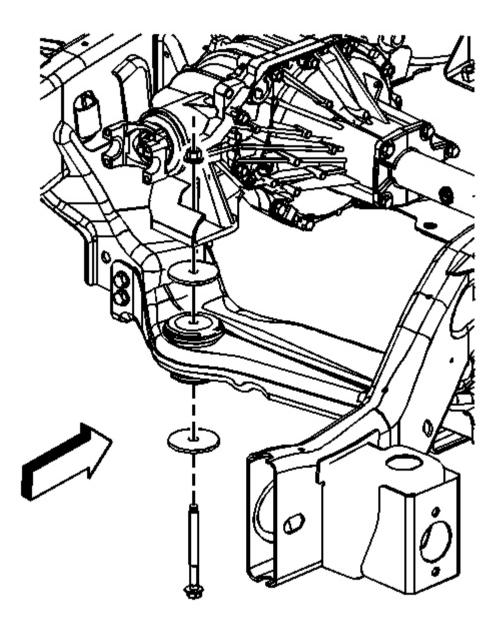
Fig. 63: Differential Carrier Assembly Left & Right Side Axle Mount Bolts & Nuts Courtesy of GENERAL MOTORS CORP.
