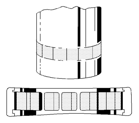
Fig. 19: Brinelling Courtesy of GENERAL MOTORS CORP.
