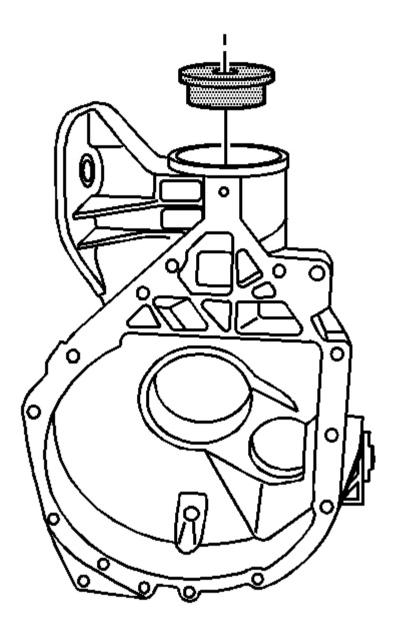
Fig. 109: Installing J 45754-1 Over Outer Pinion Bearing Cup Courtesy of GENERAL MOTORS CORP.
