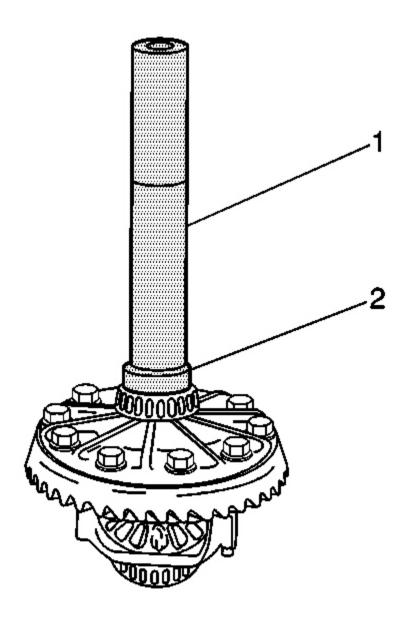
Fig. 104: Driving The Differential Case Bearing Onto The Case J 8092 & J 22761 (8.25 Inch Axle)
