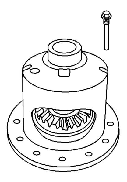
Fig. 94: Pinion Shaft Lock Bolt Courtesy of GENERAL MOTORS CORP.
