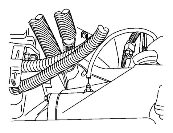
Fig. 36: Front Drive Axle Vent Hose & Vent Hose Connector Courtesy of GENERAL MOTORS CORP.
