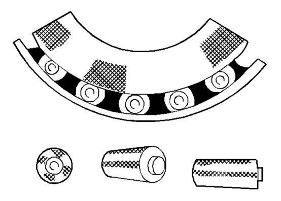
Fig. 3: Abrasive Step Wear Courtesy of GENERAL MOTORS CORP.
