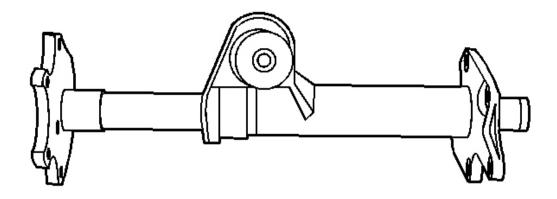
Fig. 134: Install Inner Axle Shaft Into Inner Axle Shaft Housing Courtesy of GENERAL MOTORS CORP.
