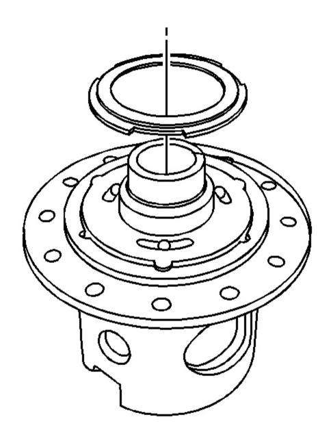
Fig. 41: Outboard Locking Differential Ball Bearing Plate Courtesy of GENERAL MOTORS CORP.
