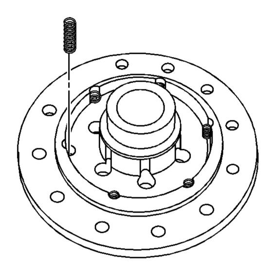
Fig. 37: Locking Differential Clutch Springs Courtesy of GENERAL MOTORS CORP.
