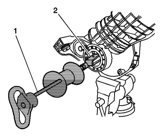
Fig. 46: Installing J 29369-2 Behind Inner Axle Shaft Seal Or Inner Axle Shaft Bearing Courtesy of GENERAL MOTORS CORP.
