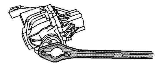
Fig. 82: Installing J 8614-01 Onto Pinion Yoke Courtesy of GENERAL MOTORS CORP.
