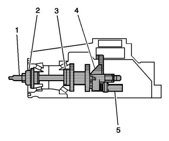
Fig. 110: Assembling J 29763 To J 36601-3 & J 36601-7 Courtesy of GENERAL MOTORS CORP.
