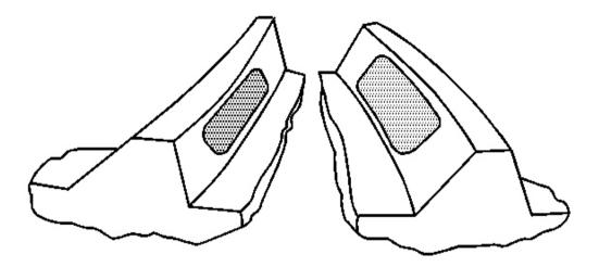
Fig. 139: Correct Contact Pattern Courtesy of GENERAL MOTORS CORP.
