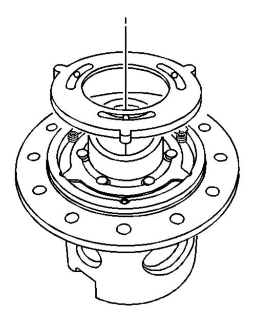
Fig. 39: Inboard Locking Differential Ball Bearing Plate Courtesy of GENERAL MOTORS CORP.
