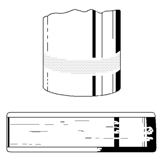
Fig. 24: Frettage Courtesy of GENERAL MOTORS CORP.
