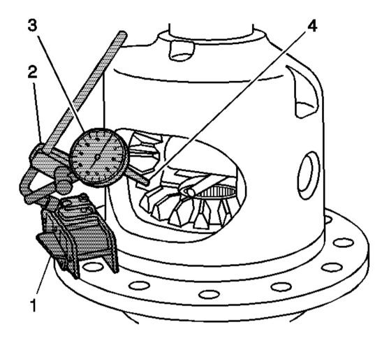
Fig. 26: Measuring Backlash Of Pinion Gear Closest To Pinion Shaft Lock Bolt & Locking Differential Side Gear Courtesy of GENERAL MOTORS CORP.
