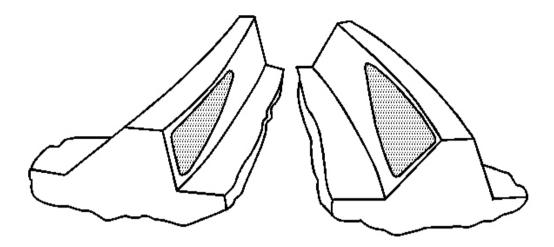
Fig. 142: Drive Side Heel - Coast Side Heel Contact Pattern Courtesy of GENERAL MOTORS CORP.
