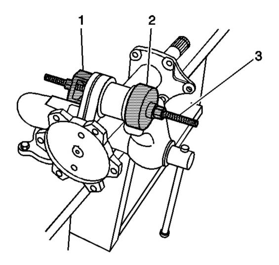
Fig. 61: Installing J 45755-2, J 45755-1, Forcing Screw, Bearing & Washers Inner Shaft Housing Bushing
