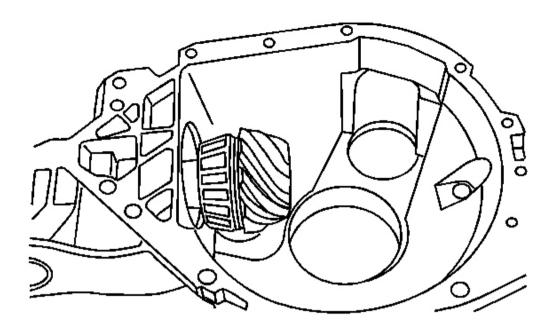
Fig. 116: Applying GM P/N 12346004 Sealant To Splines Of Pinion Yoke Courtesy of GENERAL MOTORS CORP.
