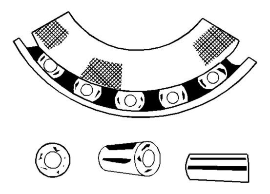
Fig. 4: Galling Courtesy of GENERAL MOTORS CORP.
