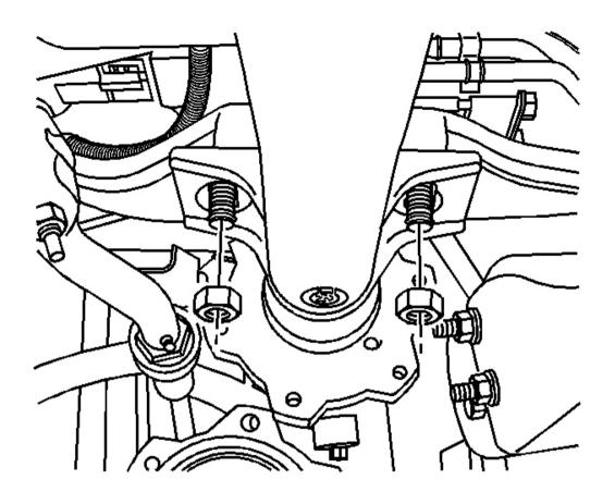
Fig. 39: Front Drive Inner Axle Shaft Housing Nuts Courtesy of GENERAL MOTORS CORP.
